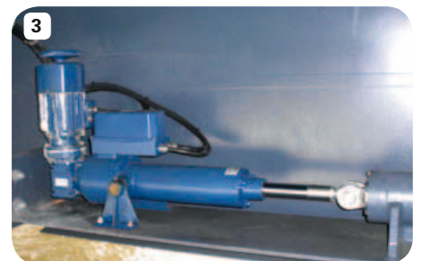
Verrouillage de pont-levis, type K1N7, course = 200 mm
